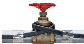
This is an electrical cable that is attached to the pipe; the cable is then wired to a transformer and attached to the electricity supply. The pipe and cable are then covered in pipe insulation and the cable is turned on and off by an external frost thermostat, normally when the temperature falls below 2.5°C to 3°C. This is effectively placing the pipe in its own mini electric blanket, warm enough not to freeze but not warm enough to heat the water above 2.5°C.
