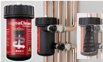
This works by using the magnetic properties of the iron oxide to 'capture' the crystals as they form. The filter is placed in the central heating system and water is allowed to flow through the filter constantly, any crystals in the water are slowly collected by the filter.
