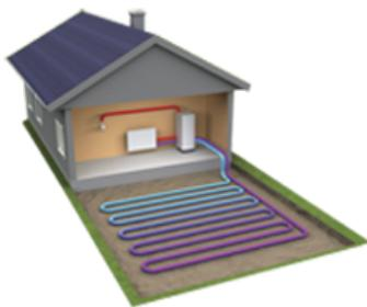
Ground source heat pumps tap into the heat energy supplied by the sun. Imagine the earth as a huge solar collector, absorbing heat energy from the sun all year around. Of course the surface of the earth is also susceptible to heat losses through weather, for example rainfall. However, the deeper we dig the more stable the temperature becomes at around 8-10°C.
