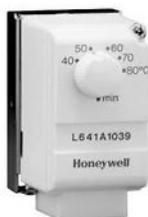
**Cylinder thermostat** - This little box sits on the hot water cylinder about 1/3 from the top. It measures when the water in the cylinder is warm enough (depending on what you set it to). As the cylinder cools down it will tell the programmer to turn it back on again.
