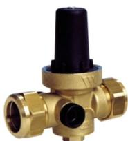
**Pressure reducing valve** - This is placed on the incoming cold water main pipe to the hot water system to reduce the water pressure slightly and keep it at a constant level of pressure.
