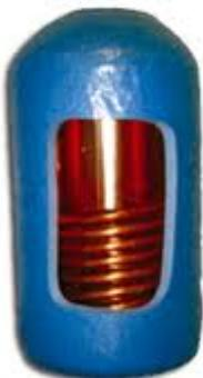
**The cylinder** - is the main part of the open vented hot water system; this is where the hot water is heated. The heat can come from an immersion heater, directly from a boiler or indirectly from a boiler using a coil fitted inside the cylinder. Often the indirectly heated cylinders come with an immersion heater back up in case of a boiler breakdown.
